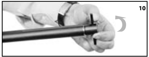
(figure 11) Choke being installed in barrel loading
