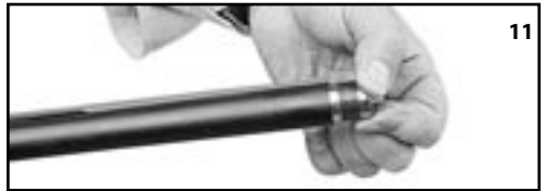
(figure 11) Choke being installed in barrel loading
