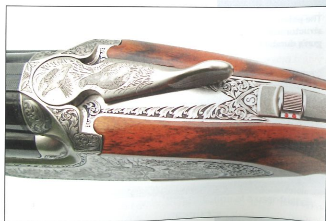
BELOW RIGHT The barrel selector combines the necessary properties of being easy to use on purpose and impossible to use accidentally
